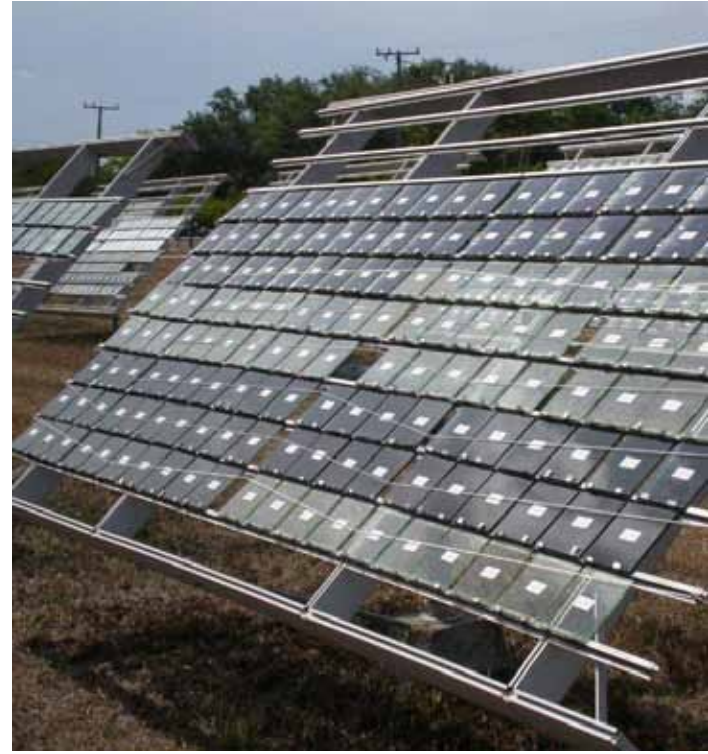
Figure 4: Exposure testing conducted in Miami, Florida, USA.
