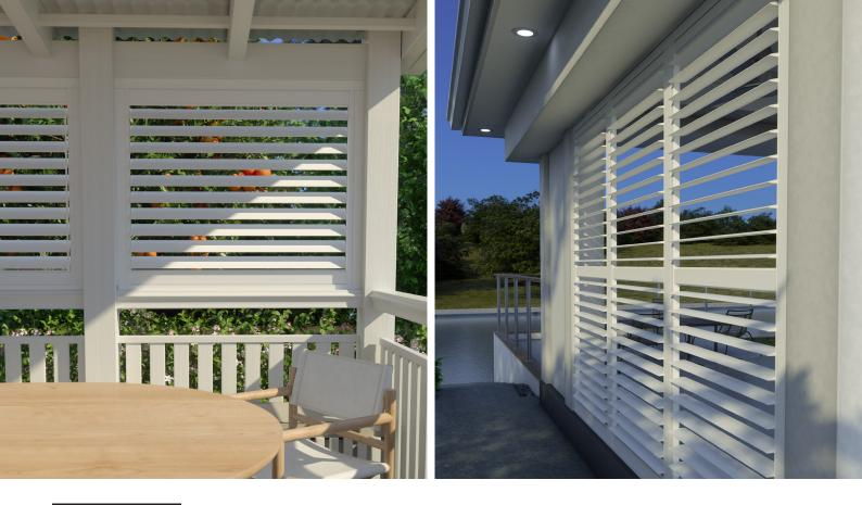
Nirvana aluminium fixed panel operable louvre shutter system features horizontal elliptical blades which can be opened or closed by tilting up or down by hand. Shutters are joined by a tilt rod allowing the blades to move in unison.
